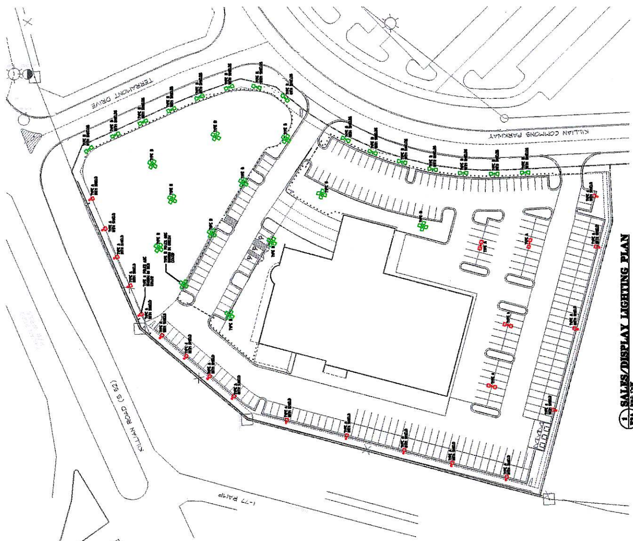
2. TYPE A FIXTURE DETAIL TYPE A FIXTURES ARE INSTALLED ALONG THE PERIMETER AND INSIDE PARKING AREAS.
